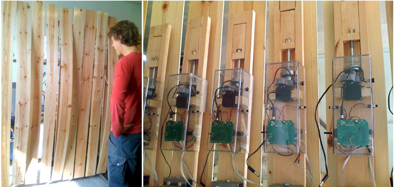
Figure 3: First picture shows the PLANKS in action. Second picture shows a close up of the computational layer and the "adhesive layer" including the motor (Unfortunately, the prototype illustrated here turned out to have a construction error and it only worked for a short while. New ones are being build.)
