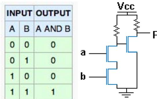
Figure 1: Example of a circuit structuring the logic AND operation—only if both a and b are high (represented by 1) will the circuit measure a high voltage level, courtesy of Wikipedia
